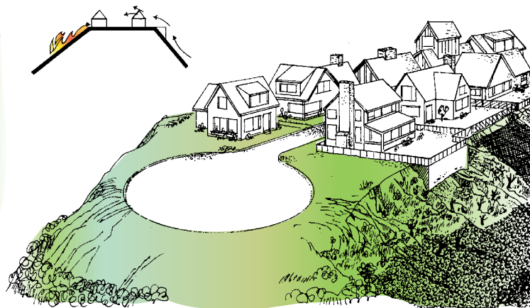
Figure 4. On narrow ridges, homes without adequate setbacks, such as those on the left, are particularly vulnerable to fire.
