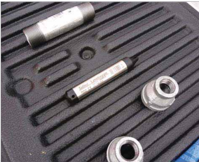
Photo 4: Water level data logger components and protective housing
