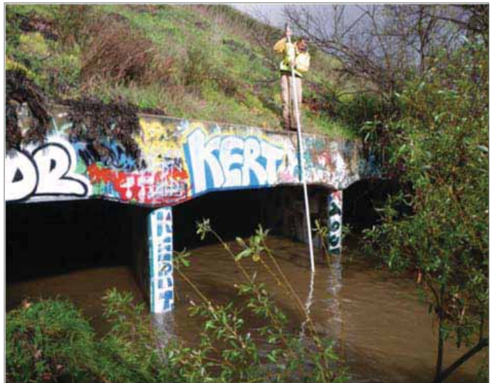
Photo 2: Stadia rod used to survey cross sections
