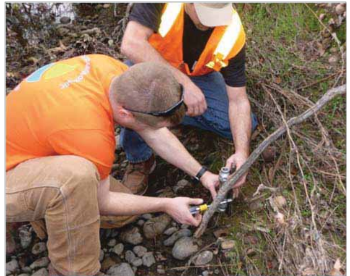
Photo 5: Field installation of water level data logger
