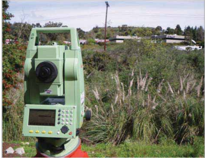
Photo 1: GPS Total Station used to survey cross sections
