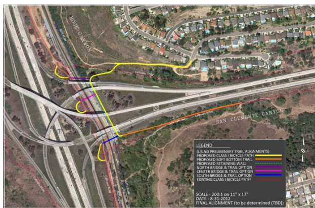
A proposed map of alternate locations of the bridge that could safely transport cyclists and pedestrians over the rail corridor beneath the I-5/SR-52 interchange. Click to enlarge
